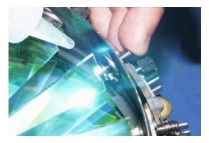
The filter carrier should spring back out on it's own. If necessary, pull the filter carrier back out of the bulkhead assembly. (Pushing the flat surface on the filter side of the filter carrier may help on some of the more difficult ones.)
