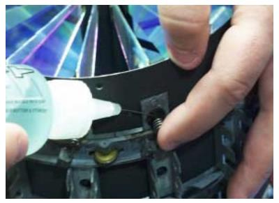
**4.** Push the filter carrier into the bulkhead assembly. It should move about 1/8". Spray some cleaner into the inside gap that has been created. See photo below.
